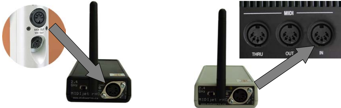
Instrument's MIDI OUT connected to MIDIjet Transmitter (black box)
