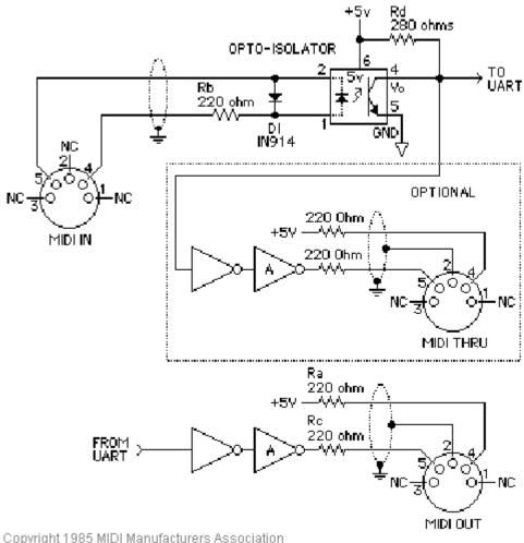
Figure 3: Schematic of 5-pin 180° DIN connections
