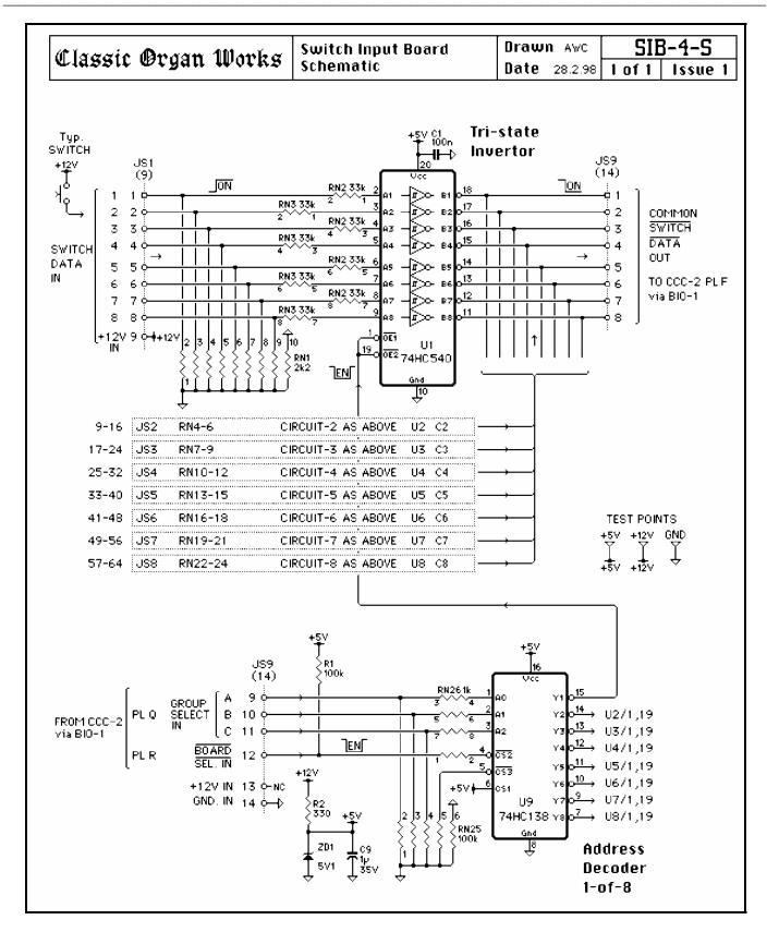
Figure 19: SIB-4 Schematic
